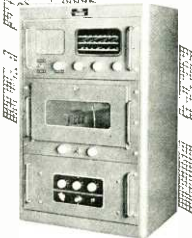
Model RGA 633 enclosed rack type Radio-amplifier equipment. Combines amplifier with radio and 3-speed record changer.
