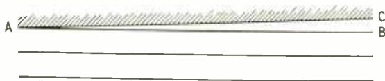
Fig. 4. The line AB represents an ocean wave rolling in towards a sea wall AC. During the time the wave takes to cover the distance from B to C, the splash on the wall has travelled from A to C.
